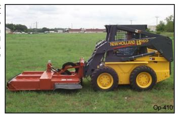
To avoid overturns, drive the skid steer with care and at safe speeds, especially when operating over rough ground, crossing ditches or slopes, and turning corners. Use extreme caution when operating on steep slopes. Travel at a slow speed when going downhill. DO NOT coast or free-wheel downhill.
